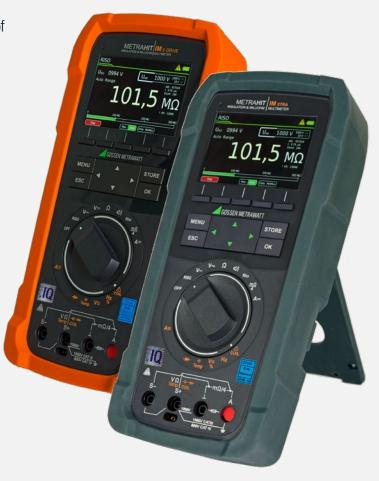
Multimeters – Portable and Compact, for More Safety in Aircraft The so-called KELVIN measuring method is implemented in measuring instruments for bonding and wick tests, i.e. a 4-wire measuring method (voltage-correct measuring method). All contact and measurement cable resistances are compensated for by this measuring method, because these would otherwise distort the final measured values. Point-to-point, point-to-structure or reverse current measurement is used.
