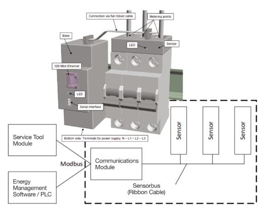
Figure 2: Diagrammatic representation of EnergySENS monitoring system
