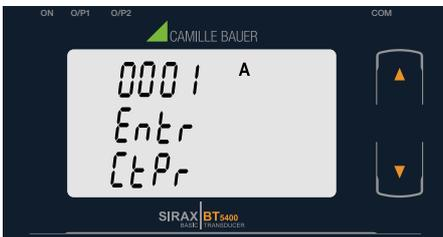
Pressing the “ Down” key will enter the transducer into “CT Primary value edit” mode.
