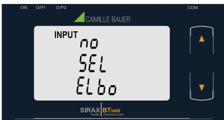
Pressing the “**Down**” key will enter the “Elbow enable or disable edit” mode and scroll the value between yes and no.
