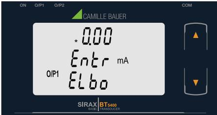
Pressing the “
