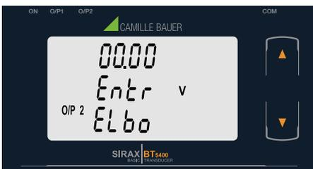
Pressing the “**Down**” key will enter the “ Output 2 Elbow value edit ” mode.
