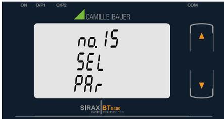
Pressing the “**Down**” key will enter into the “Parity & stop bit edit” mode and scroll the value between
