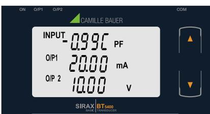
For Power Factor Transducer Input Power Factor, Output 1 as Current or Voltage
