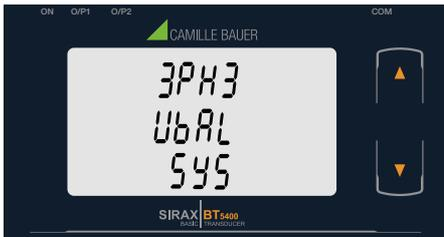
Pressing the “**⬇** Down” key will enter into the “System Type edit” mode. For Active / Apparent / Reactive Power Transducer, System type will scroll between
