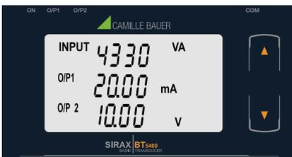
For Apparent Power Transducer: Input Apparent Power, Output 1 as Current or Voltage
