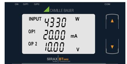
For Active Power Transducer, Input Active Power, Output 1 as Current or Voltage
