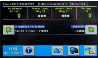
DisplayColor LCD with LED backlightResolution480 x 272 pixelsSuitable for use in sunlight
