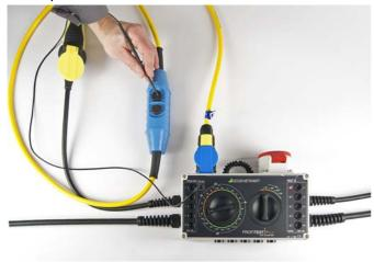
Measurement of protective conductor current for a connected PRCD using the METRACLIP 61 current transformer clamp as an accessory
