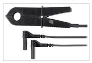
Current clamp sensor for leakage current, selectable measuring ranges: 1 mA ... 15 A, 3% and 1 A ... 150 A, 2% Transformation ratios: 1 mV/mA, 1 mV/A
