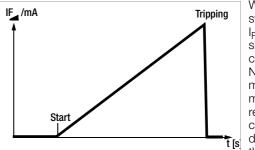
With the selector switch in the I<sub>F</sub> position, slowly rising DC current flows via N and PE. The momentary measured current value is continuously displayed. When the RCCB is
