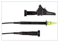
The KS24 cable set includes a 4 m long extension cord with a permanently attached test probe at one end and a contact protected socket at the other end, as well as an alligator clip which can be plugged onto the test probe.
