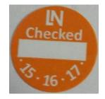
The year of manufacture/shipment and the inspector's initials appears on this test seal.
