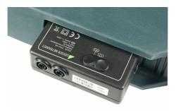
Figure 1: Leakage Current Measuring Adapter at the PROFITEST MXTRA
