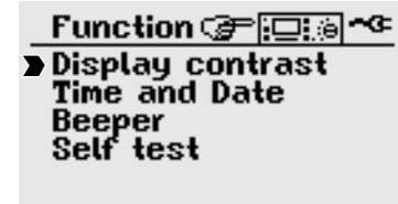
All setting and changes entered to the menu accessed in the SETUP switch position are saved to memory automatically, and are retained after disconnecting the device from mains power.
