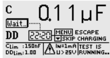
After capacitance has been determined, the instrument automatically continues with dielectric discharge testing. This takes about 30 minutes. However, the measurement can be aborted at any time by pressing the MENU key. Only capacitance is displayed in this case.
