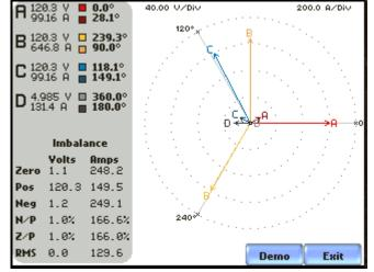
This condition would be quite unusual in the supply network. But this can also be caused by: Not completely closed current clamp jaws or weak/empty battery with active current probes or wrongly selected measuring range of the current probe. To test this, you can try to put all the current probes around the same phase conductor and compare their measured values.
