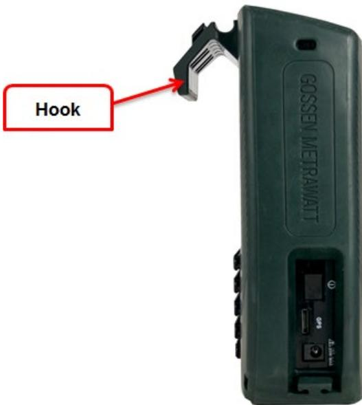
Integrated cable management is available for the user to neatly and safely 'dress' the voltage and current measurement cables by securing them to the instrument. Wire retainers are available on the instrument hanger, as well as a unique cable guide system that is available on the instrument stand.
