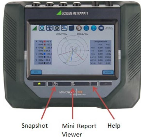
All MAVOWATT 2XX instruments have 3 'hard' buttons located beneath the LCD display. These buttons are for reporting and help functions that are available to the user at all times, regardless of the user interface screen being displayed.
