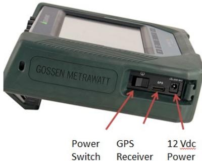
External 90VAC-265VAC, 50/60HZ, 12V output universal power supply. US, UK, Euro, and Australian country plugs are included. A user accessible NIMH rechargeable battery (UPS) is included with a 2hr (3hr for MAVOWATT 230 & 240) run time on a full charge. Charge time for a depleted battery is 3hrs.
