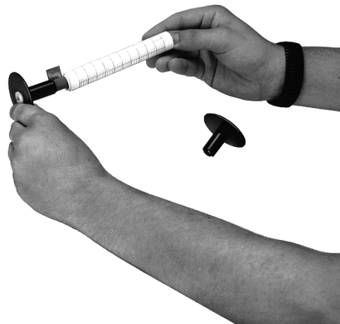
Figure 11 Removing the recording chart from the take-up roll
