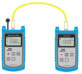
Connect the light source and the level meter KE8000 with a high-quality optical measuring cable.
