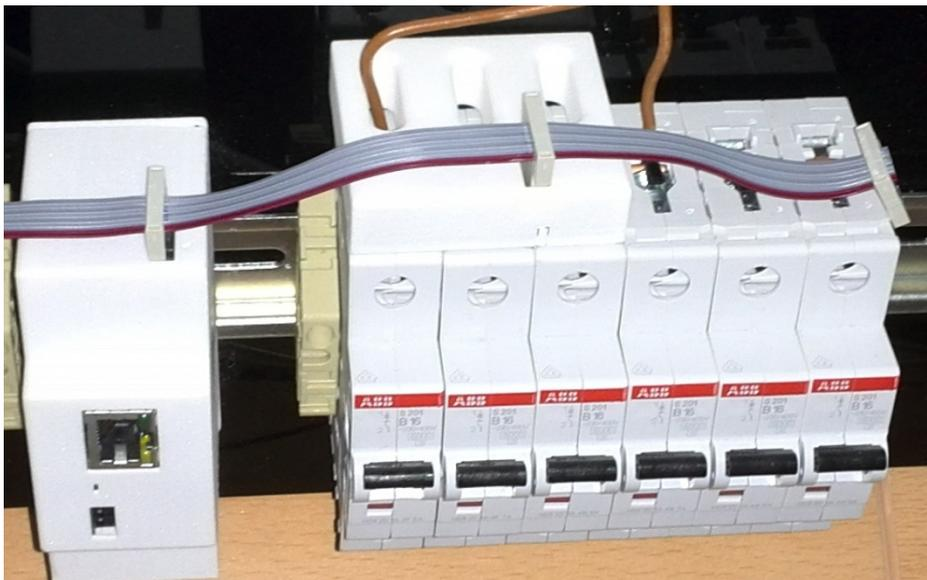
The base and all sensors are connected with a flat ribbon cable. As shown in the picture, the plugs are put in the Sensorbus interfaces of the base and of the voltage sensors:
