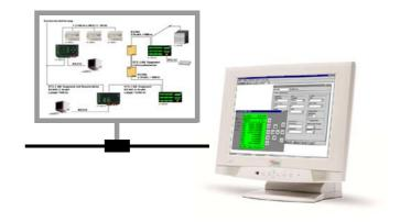
**ECSwin** is primarily used for configuring parameters for type U16xx summators in an Energy Control System (ECS-LAN). Beyond this, read-in and visualization of energy consumption data in the form of measured value tables and graphics is supported as well.
