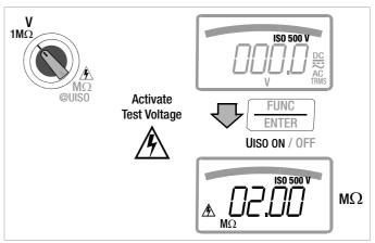
Auto-ranging is active during insulation resistance measurement.
